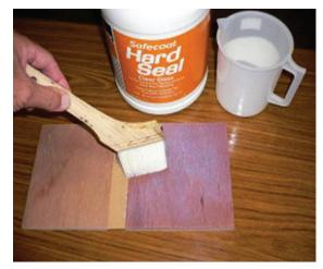
Safecoat Hard Seal is applied to the right side of (bad) plywood. 3 coats. The left side is left uncoated.
