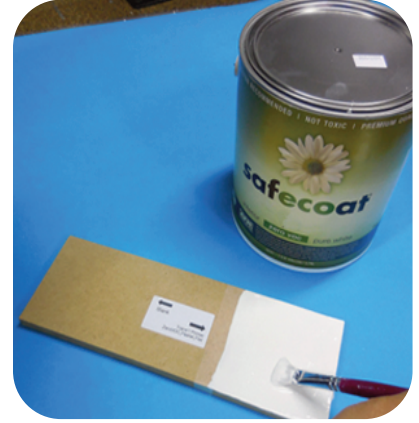
Another coat was applied two hours later with same coverage.
