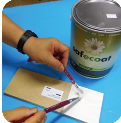
Safecoat Zero VOC paint was applied a day later with same coverage.
