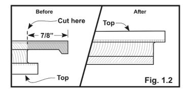
1.3 Set saw depth to cut off these protrusions, being careful not to cut too deep into bottom of wearlayer.
