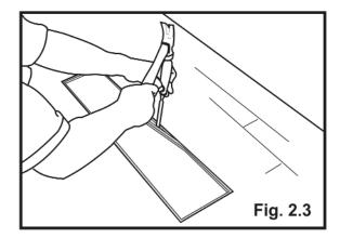
2.3 Carefully remove remainder of board still attached to adjacent boards using a chisel and hammer as shown in Fig. 2.3.
