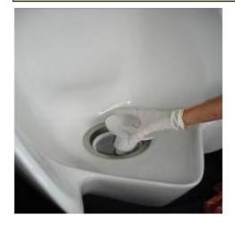
Take a new Drain Insert and place it in the waste trap.
