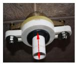
Lubricate drain tube and Run in and out until this can be done easily.
