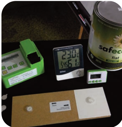
One week later, formaldehyde emissions were tested with NTE-3100 and F.R.A.T. method 0917-1. Emissions can be read via either Desiccator (mg/L) or Small Chamber ( \mu\text{g}/\text{m}^2/\text{hr} ) methodology.
