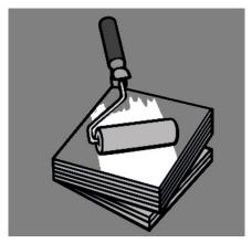
**STEP 2:** Apply thin coat of adhesive evenly to the entire back of cork tiles. Allow to flash off for approx 60-90 min.
