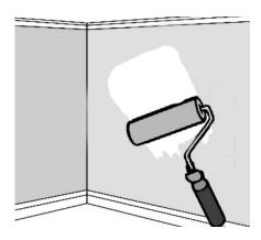
STEP 3: Stir adhesive well. apply to wall with roller or trowel and allow to dry approximately 30-45 min.
