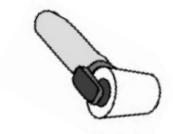
**STEP 5:** Apply pressure with your hands, and then a rubber mallet or roller to ensure pressure is applied evenly.
