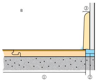
3. Movement joint x 1.5 = skirting board minimum thickness in mm
