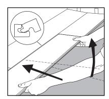
**STEP 4:** Place short end of plank at an angle to the first board. Lower down and then angle plank against first row.
