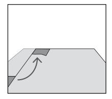
**STEP 3:** Cut the final plank with utility blade or saw and use the leftover plank to start the second row.
