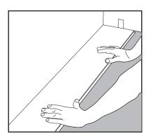
**STEP 1:** Begin installation from right to left. Insert spacers at ends and edges to maintain a gap of .2"
