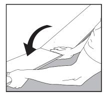
**STEP 2:** Lock short end of plank by inserting tongue into groove at an angle and drop in place. Complete the first row.
