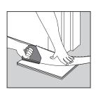
If a door frame needs to be cut, use a piece of plank to obtain the correct height. Always check with local codes for government or multi-family buildings.
