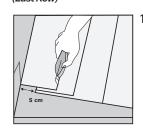
Measure and cut the planks in the last row to the correct size.
